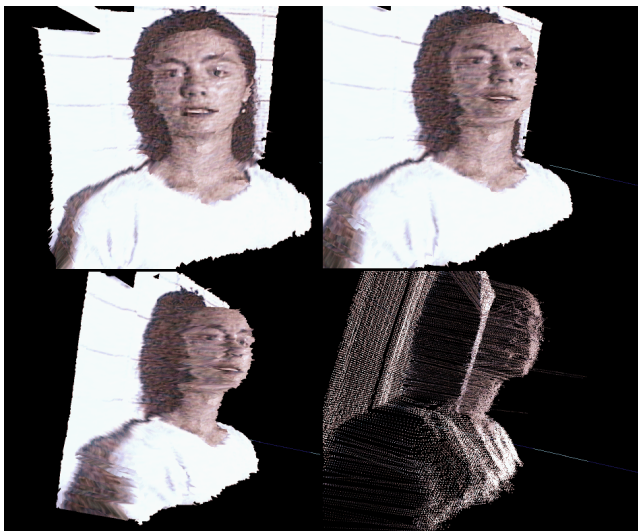
Figure 3: Some example results (still frames from live updates) of depth extraction using binary coded structured light.
